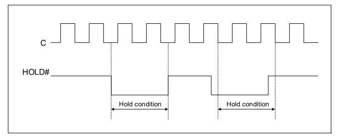
The Hold condition starts when the Hold (HOLD#) signal is driven low when Serial Clock (C) is already low (as shown in Figure 5-1).
